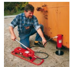
Lifting of a container by use of an hydraulic cylinder YS-23/160, lifting claw AYS-23 and piston plate AYS-232 powered by a two-stage hand pump HPS-2/2 with base frame HPB-2.
